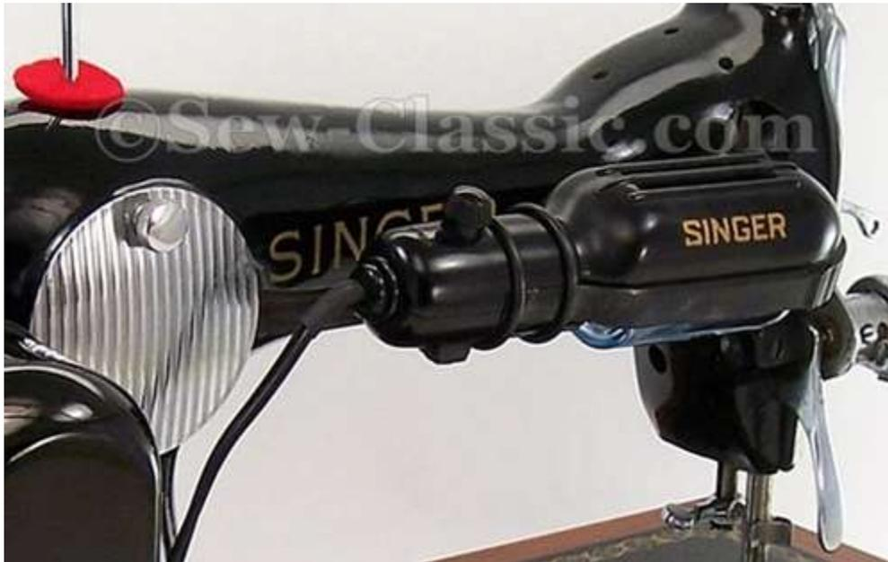
The first type shown is the most difficult of the two to open up and rewire and they often have worn contact springs. The only source I know of for replacement contacts is from another old fixture. To open this first type, you have to spread apart the three metal compression rings. It's a bear to do, but not nearly as big of a pain as getting it back together. My best advice is to curse softly so as to not offend the neighbors. Also, keep band aids handy.
