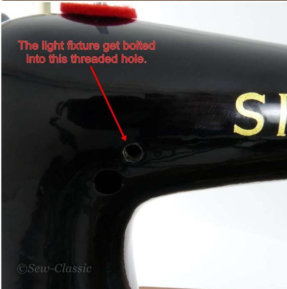
The light fixture get bolted into this threaded hole.
