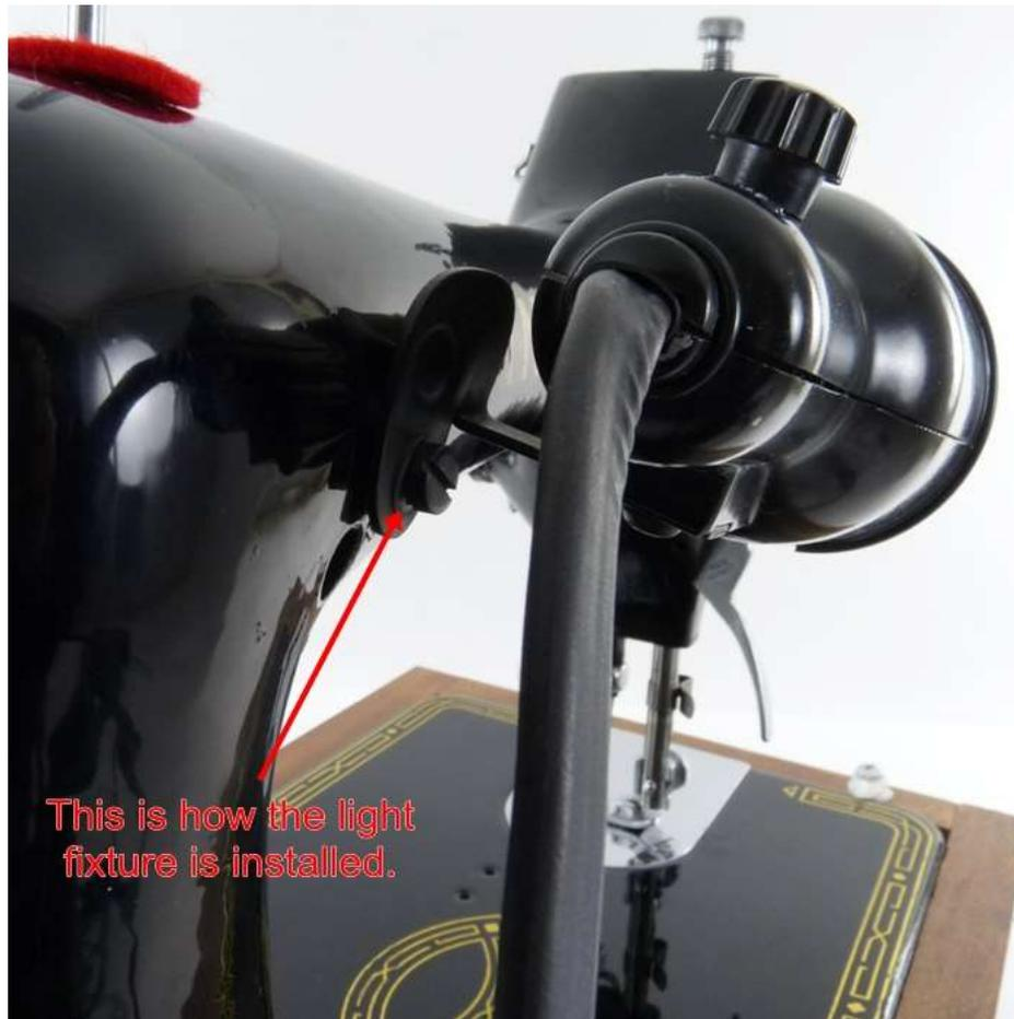
This is how the light fixture is installed.
